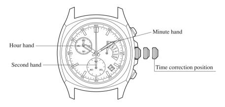
In the case the crown is of the screw-lock type, loosen the screw by turning the crown to the left before operating the crown, and after having returned the crown to the normal position following operation, turn the crown to the right while pushing it in to securely retighten it.
