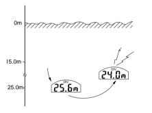
**1. Ascending Speed Warning** If the ascending speed exceeds 1.5 m (5 ft) in 10 seconds during a dive, the alarm will sound for more than 10seconds as the ascending speed alert.
