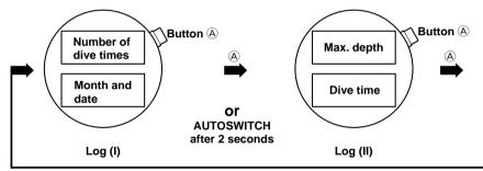
• Each time button (A) is pressed, the log display is changed to the next in the order of (I), (II), (III) and (IV).
