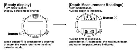
When a depth of 1 m (4 ft) is reached after you begin diving with the watch displaying [Ready display], the display will automatically change to [Depth Measurement Readings].
