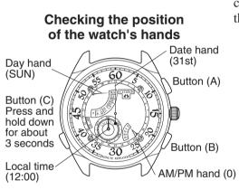
Positioning of the watch's hands... This feature allows you to check and<br/>confirm the proper position for each of<br/>the watch's hands.
