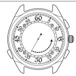
• When the date hand quick-advances in a counterclockwise direction this indicates that the initial setting was not successfully completed. See "15. INITIAL SETTING" for further instruction. (Initial Setting incomplete warning indication)
