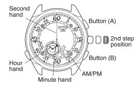
(4) When the Sub watch second hand is not aligned with the "0 sec" position, press (A) button to set it to this position.
