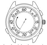
• When the date hand quick-advances in a clockwise direction this indicates that the "time setting" between the Main watch and Sub watch was not successfully completed.
