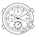
If the watch is put in the undercharged state during any display mode, it switches to the time display when in other display modes, then the second hand moves to the ▲ CHARGE position, indicating insufficiently charged.
